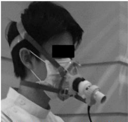
Note: The gas mask was secured to prevent breath leakage. The masks were adjusted to enable breathing through the gas mask.
